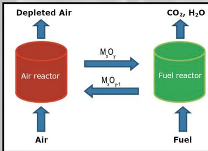
Oxygen carrier (OC) is a material composed of one or multiply metal oxides. It is capable for releasing oxygen in certain conditions, as when changed oxygen partial pressure. OCs are used in Chemical Looping Combustion technology (CLC), for transporting purposes of oxygen from an air to fuel reactor. Therefore, an oxygen released from OC structure is used to combust a fuel. That approach is significantly competitive to fuel combustion in pure oxygen atmosphere (oxy-fuel combustion).
