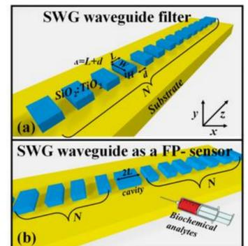
Fig. 7 SWG structure for sensing applications [5]
