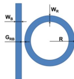
Fig. 3. Basic RR structure and parameters [4]
