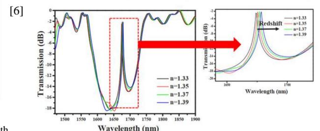
Fig. 10. 1D-PhC response for different ambient refractive indices [6]
