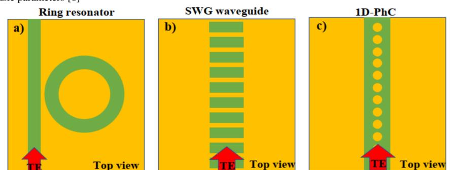
Fig. 11. Schematic representation of different refractive index sensing waveguide structures: a) ring resonator, b) subwavelength grating, c) 1D photonic crystal [1]
