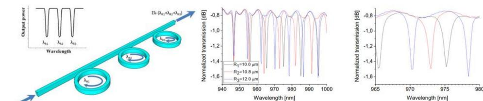
Fig. 5. Three RRs in serial operation [4]
