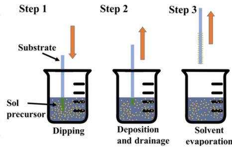
Fig. 1. Fabrication process of  $\text{SiO}_2:\text{TiO}_2$  platform via sol-gel dip-coating.
