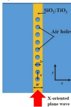
Fig. 9 1D-PhC scheme with basic parameters [6]
