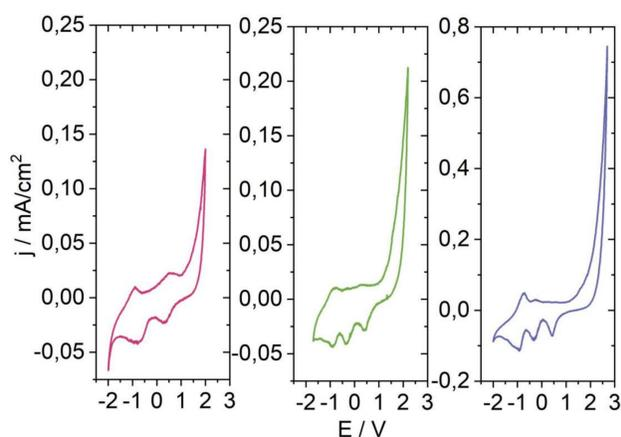
Fig. 3 Voltammetric curves registered on platinum electrode coated by thin film after the potentiostatic oxidation of naphthalene.
