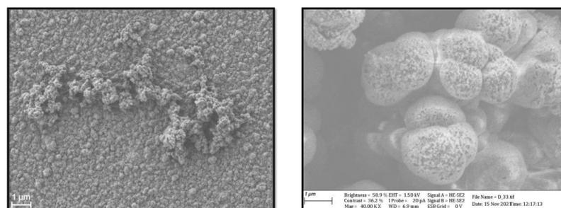
Fig. 5 Results of SEM imaging of the surface of the FTO electrode covered by the film after potentiostatic oxidation of naphthalene at concentration of naphthalene: 3mM (left), 18mM (right).
