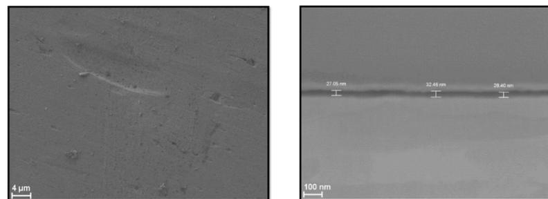
Fig. 4 Results of SEM imaging of the surface (left) and cross profile (right) of platinum electrode coated with a thin film after the potentiostatic oxidation of naphthalene.
