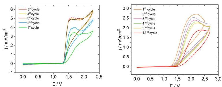
Fig. 1 Voltammetric curves of naphthalene oxidation on the platinum electrode (left), on the FTO electrode (right).
