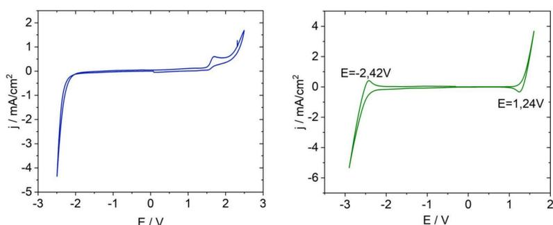
Fig. 2 Voltammetric curves registered after prior oxidation of naphthalene on platinum electrode (left), on the FTO electrode (right).
