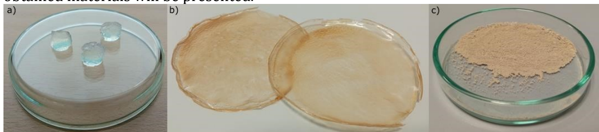
Fig. 1. Images of obtained pectin based: a) hydrogels, b) foils, c) ZnO nanoparticles
